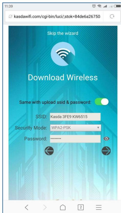
**STEP 8:** After the settings are 100% applied, the connection between Smartphone and Extender will be disconnected automatically, please reconnect to the Extender's new **WiFi network name** with new **WiFi password**, then you will have internet access through the extended WiFi Network.
